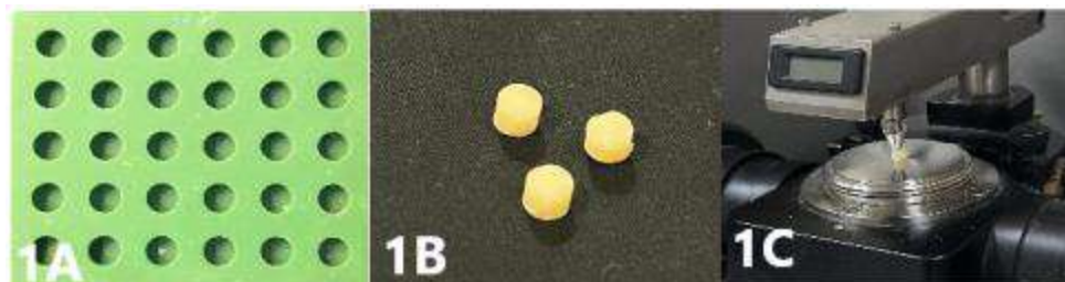
Figure No. 1: Composite resin specimen preparation and degree of conversion (DC%) assessment. (1A) Customized silicone molds (5×4 mm); (1B) polymerized bulk-fill composite specimen removed from the mold; and (1C) FTIR-ATR analysis for DC% determination.
