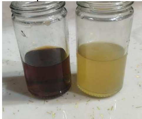
Figure No. 1: The color changing of solution to brown due to the reduced process of \text{Ag}^+ - Ag nanoparticle.
