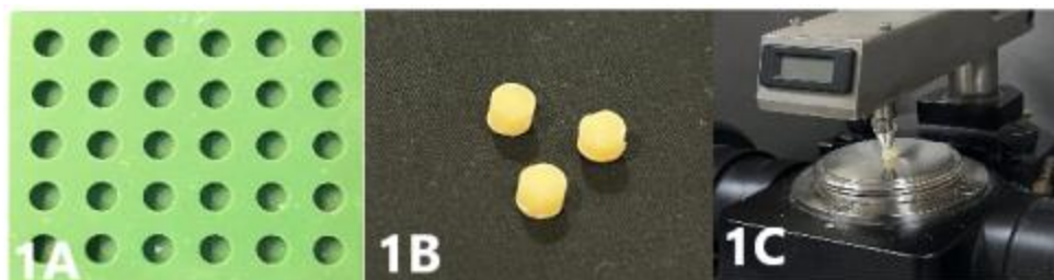
Figure No. 1: Composite resin specimen preparation and degree of conversion (DC%) assessment. (1A) Customized silicone molds (5×4 mm); (1B) polymerized bulk-fill composite specimen removed from the mold; and (1C) FTIR-ATR analysis for DC% determination.
